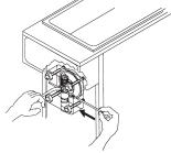
Figure S Insert Retaining Pin
